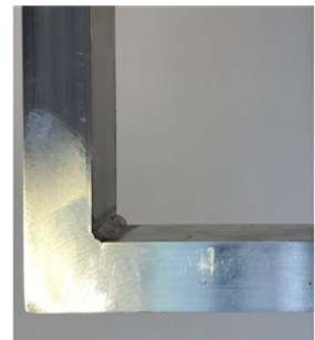
7-8: Surface grinded for smooth mounting of twin wall
