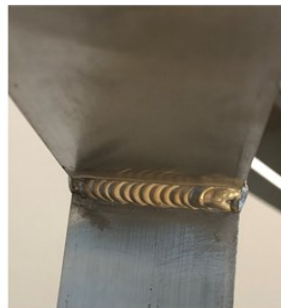
1-6: TIG welding to quality level 'C'
