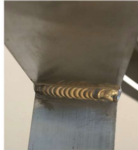
1-6: TIG welding to quality level 'C'
