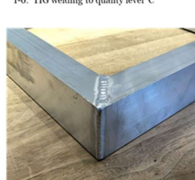
1-6: TIG welding to quality level 'C'
